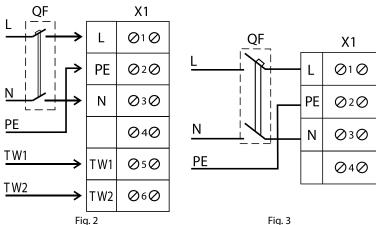
The TW1, TW2 terminals are the electrical leads of the normally closed contact of the motor overheating protection.
