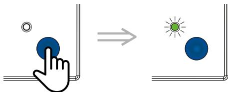
Press and hold the button until the LED starts flashing green.
